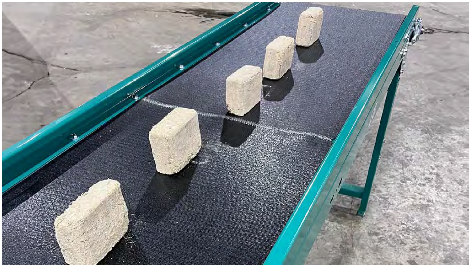
Graphyte's carbon blocks being produced at their Loblolly project site in Pine Bluff, Arkansas. Each block contains 1.8 kg of CO 2 e that are permanently removed from the carbon cycle.
